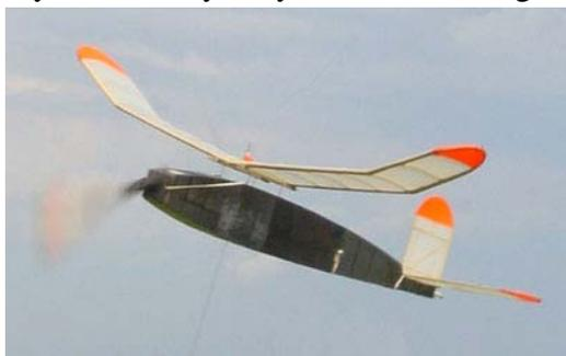
stuff. My newly tried low (no) torque approach (more later) has spread to small rubber too and the Beaver now apologises just eight strands of 3/16 Tan II from 36 grams. You can always tell when flying this method because more than half the motor hangs out front before winding commences. Piling on 14/1500 turns takes an age but the prop paddles away for about 100 secs so the trick is to get at least a bit of lift to make today's 2 1/2 minute max a possibility. The downside, of course, is if
