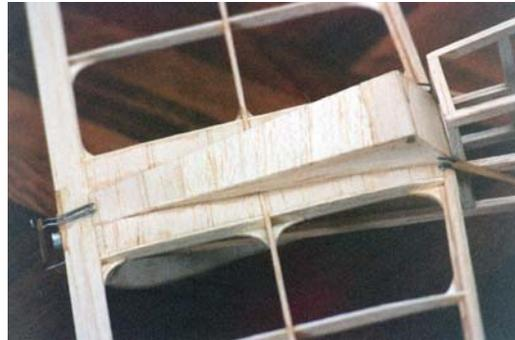
Below, is the arrangement for fixing fins to the ends of the stabilizer. The hooks are soft iron wire and the bamboo pegs locate into holes in the 1/64" ply facing on the end rib. The fin stiffeners are 1/64" ply. Fin trim tabs had to be added at the flight trimming stages. Removable fins are greatly beneficial in preventing transit damage. The stabilizer spends **ALL** its stored life on a former, as do the wings (center panels).
