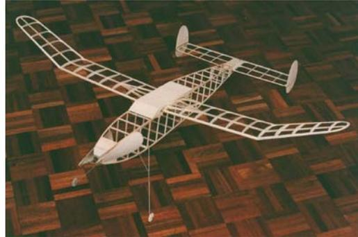
Here, the D/T leverage band pulls the stab forwards and down, to lock its angled front against the upright member of the platform. One or two rubber bands are all it takes to provide both the leverage and the lock into the D/T position. The little bamboo dowel is a slide fit into its holes and therefore removable for repairs/maintenance if required. The 1/32" soft gussets between the ribs and LE (and TE too) add strength and are sanded concave for neatness and to minimize any added weight.
