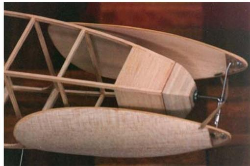
The prop blades are (were) two laminations of dissimilar wood (as can be clearly seen) molded around a 6" diameter stone jar, 15 degrees to the vertical. This eventually turned out to be a big mistake because after about 5 years the blades warped dramatically to cause serious unresolved flight problems. Eventually this was resolved by replacing the blades with carved units. The coup de gras, just about visible, are the bamboo laminated edge protections. Ah, the miracle of Cyano!
