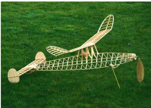
“New Look I” could hardly have been more different in design and layout. Following a line of development commenced in 1948 this version appeared in 1950 to compete in the 8oz Wakefield class. The model featured a single leg retracting undercarriage below a long diamond fuselage with a rear peg well aft, allowing for a very long motor too. It sported a tall pylon supporting a high aspect ratio poly-dihedral wing with ultra thin under-cambered
