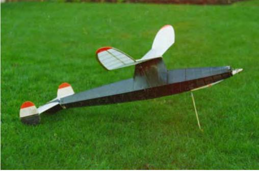
Not-with-standing, the wing was put together in one piece with the top mounted main-spar and its dihedral angles pre-constructed with very accurate scarf joints over an appropriate engineering drawing. Using two thicker centre ribs, 1/64" apart, each panel was built on to the whole spar, propping up the completed panels as work progressed. Joiner tubes made from RC snake outers were let in to the centre sections before the wing halves were separated with a
