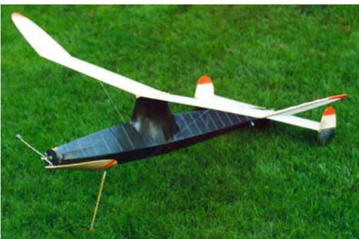
efficiency of the tailplane and originally only the right fin was removable because the other had to withstand the very high torque at take-off due to the designer using 120 grams of rubber. He maximized wing and stab areas by using caches to cover their center sections. On top of all this he introduced a lifting tailplane with positive incidence to prevent too much nose-up during the power run (In my case this proved a jeopardy too far, as described later).
