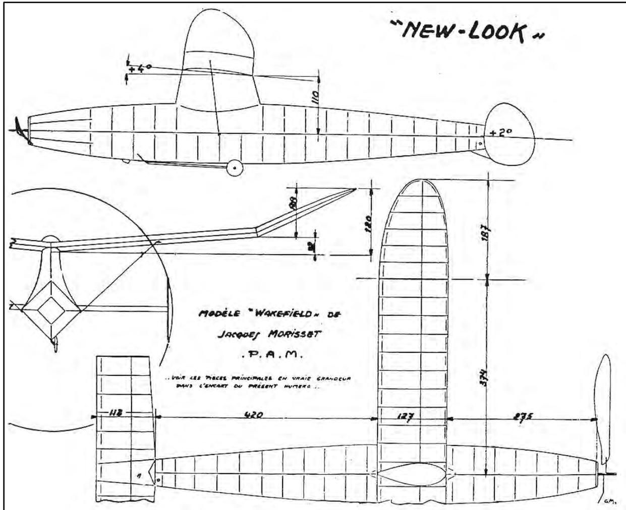
"New Look 0" was built, flown and lost at Easter '48 Team trials. It had an inverted vee tail. "New Look I" was built with the following ideas. High motor weight of 120 g, hence a long fuselage to keep the motor section down to 100 sq mm. An old rule said not to go past 50% increase over the nose to rear hook length, so this was fixed at 800 mm.
