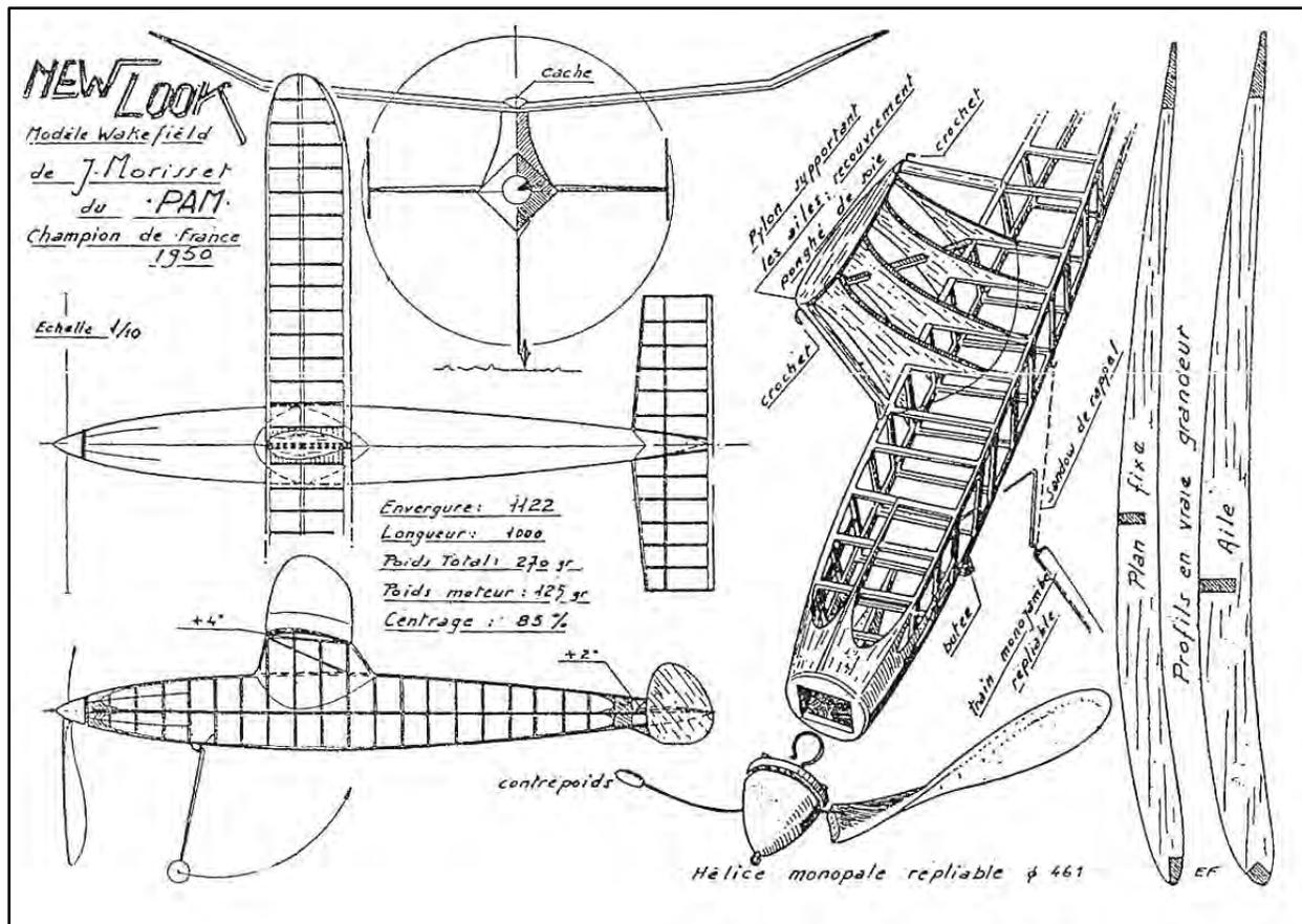
The drawings include some minor changes from the prototype. Fuselage cross section increased from 71 x 71 to 80 x 80 mm. Removal of wing centre cover. Slight shrinking of the wing to account for the non-covering of the wing centre by this cover (area: 13.48 sq dm).
