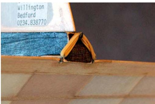
Leverage for the action is provided by two small bands around extended hooks on the trailing edge and a single hook below the fin. Positive front location is achieved by two small bamboo bumps near the leading edge either side of the fuselage. The leverage bands also provide for positive rear location by virtue of the trailing edge hook positions in relation to the platform.
