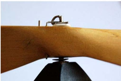
The clutch mechanism is a simple and safe design and from the image it is easy to see the single loop which catches a pawl to drive the prop. It also doubles as a winding loop. The thrust/cup washers are made from two convex drawing pin heads, the "tube-within-a-tube" bearings are brass and the Teflon
