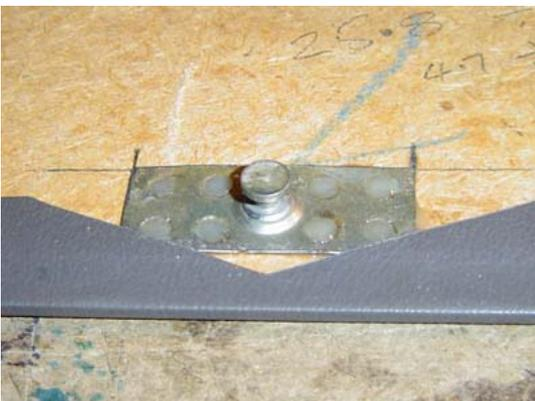
Make sure the rear face of the plate is perfectly flat and cut back part of the covering material to allow the plate to sit nicely in its new position. Mix up some regular Araldite, (not the rapid stuff, it sucks!) and work a small blob into each hole with the pointed end of a kebab stick. Also work some adhesive into the recess at the rear of the button and lightly over the rear of the plate.
