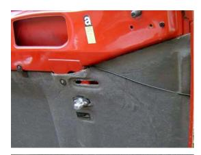
Offered up, the replacement would clearly fit exactly as Rover intended and is well supported by its six retaining clips with the sides neatly tucked into the bonnet edges. Yet, in our increasingly humid climate, for how long one wonders? Hence, to combat future shrinkage the former retaining gadgets are duly tidied up and re-fitted. The images show these fixings and their location.
