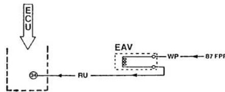
valve has closed after warm-up due to the combined effect of the heating coil and the coolant temperature being above 60 - 70°C the heat from the coil will continue to ensure that it does not open again until or unless the engine cools.
