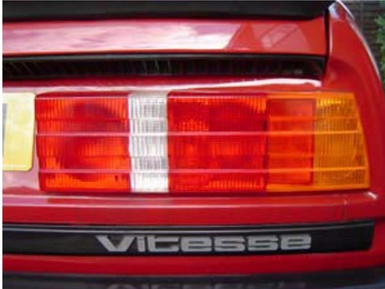
In the mid '90's the Bedford region discussed the merits of improved Rover SD1 tail lights by substituting the 21W "stop" lights with conventional 21W/5W "stop/ tail" holders/bulbs and wiring the extra "tail" filament in parallel with the existing 4W bulb, which itself can be up-rated to 5W.
