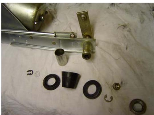
Well it's no wonder, as I just inspected my new one and found that all the external bearings are completely devoid of lubricant. Not a trace! If that is how Rover received them from the manufacturer then it was no surprise the original mechanisms wore out so badly
